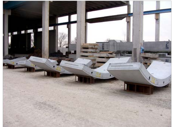
Figure 4.6: Concrete segments with stress cells and strain gages installed inside
